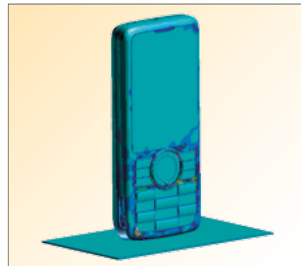
Virtual drop tests of a cell phone are performed using Abaqus to analyze the stress and strain of main parts as the phone strikes a surface from various directions. Realistic simulation enables design engineers to evaluate whether the stiffness of the phone's components meets performance requirements. Image courtesy of Lenovo.
