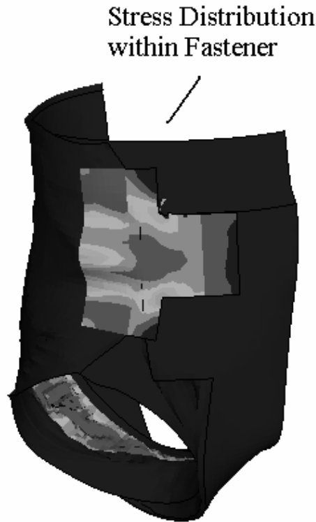
Figure 5. Stress distribution within the diaper fastener and inside view of the containment flap (baby not shown)
