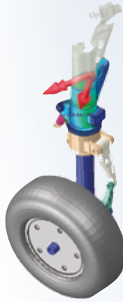
Abaqus/CAE free body diagram for an aircraft landing gear strut.
