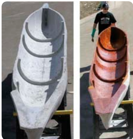
Figure 3: Meridian (left) just after removing the forms and (right) during finishing
