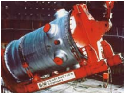
Figure 1: A nuclear reactor pressure vessel that houses the fuel rods. Exterior view of the nozzles (with red caps) through which hot and cold water circulate into and out of the vessel. (Photo courtesy of Westinghouse)
