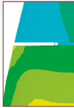
Figure 5. A side-view of EXPERT illustrates the temperature differences at the junction between the ceramic nose and the metallic after-body. The detail view (right) shows where step (radial displacement) and gap (axial displacement) measurements are made. The analysis verified that step and gap changes during re-entry fall within specifications.
