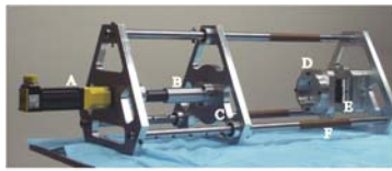
Figure 1 A pictorial representation of the CT compatible testing device. A: servo motor (SM 233, Parker Hannifin Co, CA), B: driving mechanism and C: loading platen, D: the specimen mounting ring, E: 6DOF load cell and F: Torlon™ rods.
